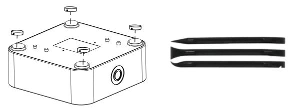
3 Remove the bottom cover of the sensor with a star-type screwdriver(T8H size).
