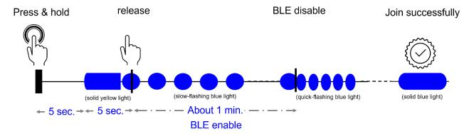
Press and hold the button for over 10 seconds until the BLUE LED starts blinking. when the BLUE LED starts blinking (like a breathing light), the DFU mode is enabled. Users can upgrade the device FW via BLE.
